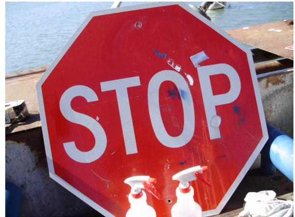
Often the public works people will try to remove the spray paint, marker and stickers and when the sign printing and color is defaced by the removal, they will simply discard the sign and replace it with a new one. The defaced signs can be sent back to the sign manufacturer and they can be reused with new screen printing, but even so, it is expensive to replace the signs so often.
