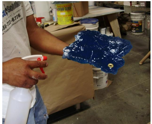
When the coatings had cured, the mats were tested on the concrete overlay mix and the concrete mix. In both cases, the bottom of the coated stamp mats retained too much residue to be practical in a field application. Many mat suppliers in the industry have sought a non-stick alternative for several years but nothing has proven successful. IRTA's testing so far has not been successful but IRTA has identified another coating that holds promise. It will be tested shortly.
